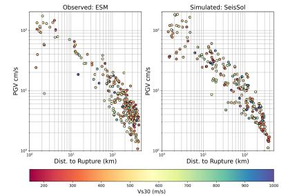
Test case application comparing observations to simulations via eGSIM
